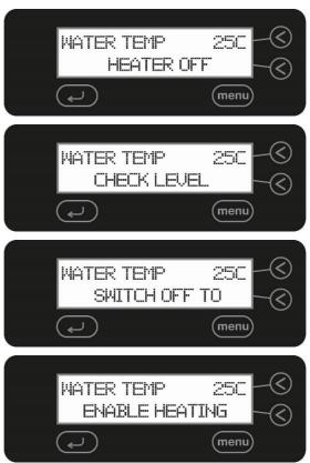
To continue using your Q-Series ultrasonic bath, refill with liquid up to the level sensor, switch the unit off and on again.
