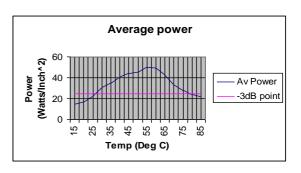
If you are using your bath to clean medical equipment, it is recommended to limit the liquid temperature to 40°C. This will avoid the coagulation of protein and other bio burden which can then bake onto the equipment.
