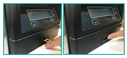
The memory card can be connected to a PC, using this memory to USB card reader to give a permanent electronic record of the cleaning parameters of the cycle.
